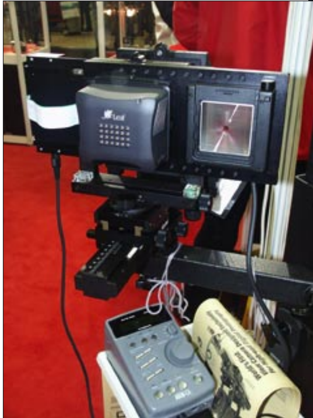
The Horseman sliding digital back holder on a 5 x 4 system. Sliding backs are not new, but this one can be controlled by computer, servo operated, and even stepped across the image field to provide a stitch-together panoramic image. It also works with film...
